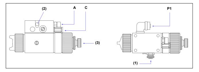
For the gun, model A 26 HTi, the base is fitted with two air needles : one for the fanned air outlet adjustment (AE  $\rightarrow$  fan width adjustment), the other one for the center air adjustment (AC  $\rightarrow$  spraying fineness adjustment, according to the the gun fluid output).
