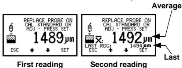
**Figure 29. Step 1 - Calibration adjustment on thickness standard**
