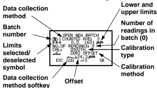
**Figure 47. Second OPEN NEW BATCH screen - Immediate mode**
