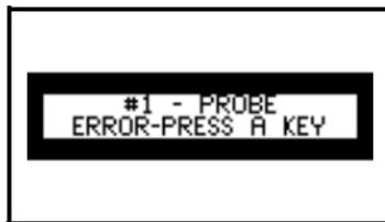
**Figure 56. Example error message - no probe is connected to gauge**
