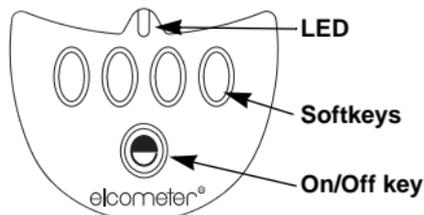
Figure 3. Elcometer 456<sup>3</sup> control keys
