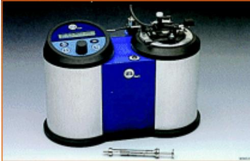
Elcometer 6910 Setaflash “Series 3” Closed Cup Tester
