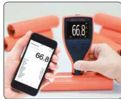
Transfer live data via Bluetooth® 2 to PC, Android™ or iOS mobile devices.
