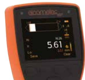
In scan mode the gauge takes readings at a rate of 16 Hz (16 readings per second).
