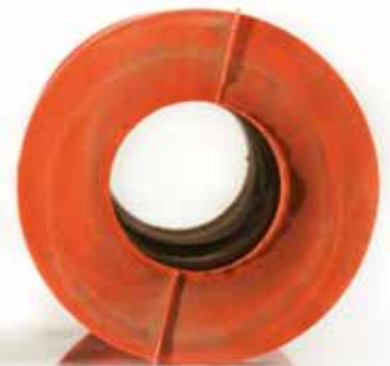
elcoTOUGH™ Valve Liner after 1665 hours using copper slag at 8bar (116psi)
