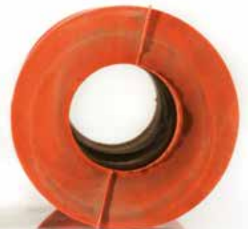
elcoTOUGH™ Valve Liner after 1665 hours using copper slag at 8bar (116psi)
