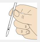
4. Insert sleeve with extract 5. Immediately remove solution and titration tube and read the number on into the hole previously the titration tube at the made in the box lid and interface of the colour change. Pink is normal, white is the chloride level.
