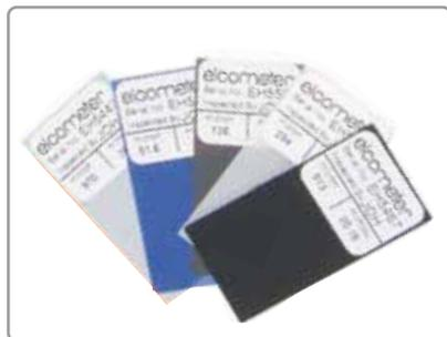
Calibration foils or 'shims' are the most convenient way of creating a coating thickness standard on the substrate material, surface finish or form. This is the ideal method for adjusting the calibration of the coating thickness gauge to ensure the greatest possible accuracy.
