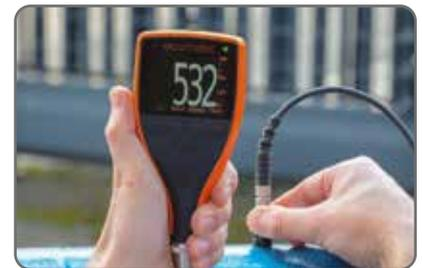
Halve the inspection time using the scan probe
